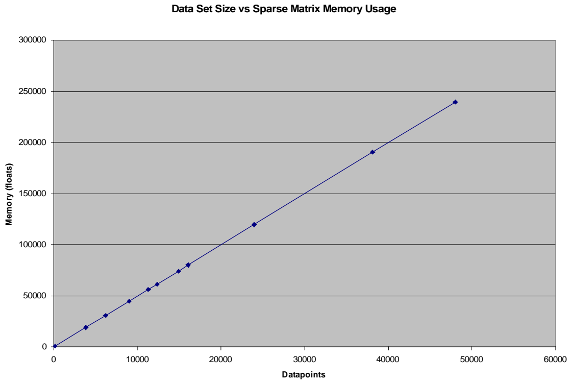
Fig. 9 – Data Set Size vs. Raw Memory Usage. As expected, memory requirements do grow linearly.
